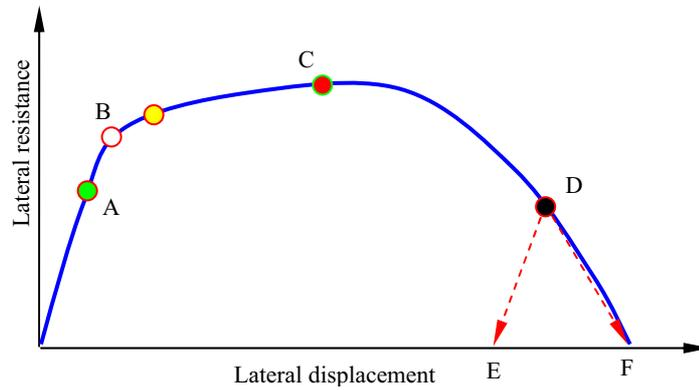
Fig 11 Lateral-load resistant behavior of structures
