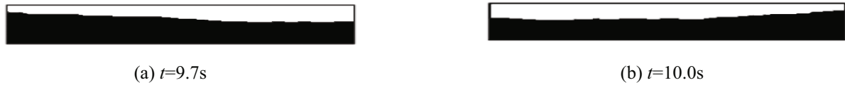
Fig. 4 Vibration of the liquid free surface (Natural freq.= 1Hz, Max amplitude = 0.05m)
