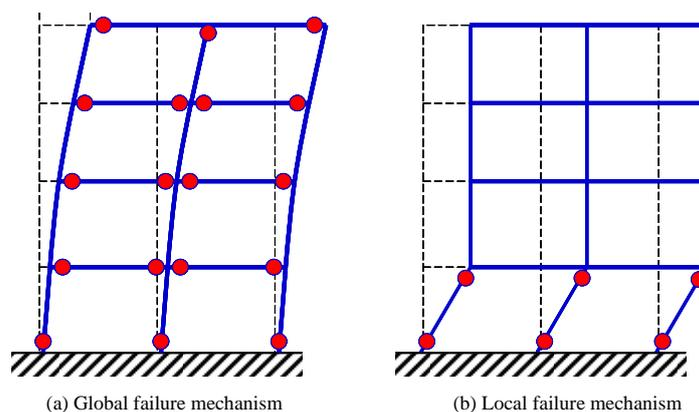
**Fig.3** Failure mechanisms of structures with “strong column-weak beam” design
