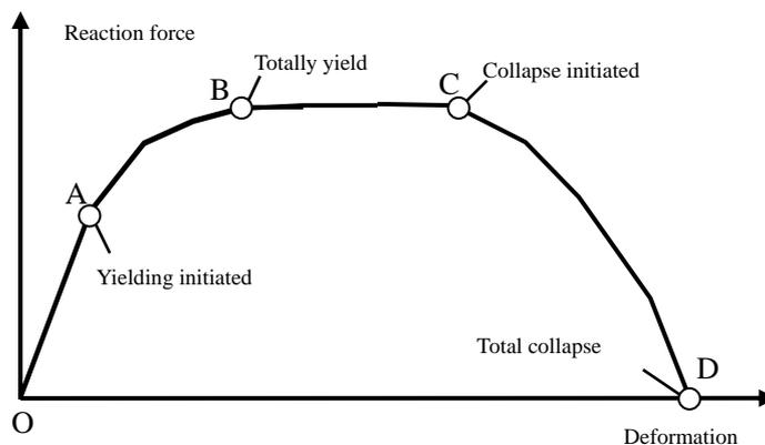
Fig.1 Desirable seismic performance of building structures
