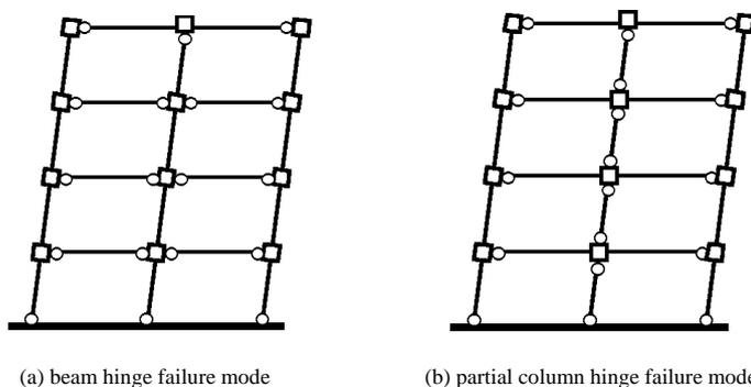
**Fig.4** Two global failure modes for frame structures
