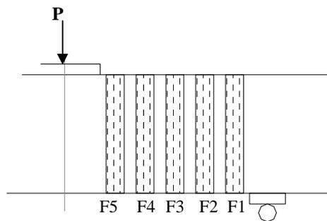
**Fig. 2.** Strip notations along the shear span
