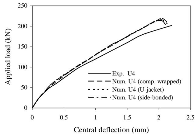
**Fig. 6.** Comparison of load–deflection relationships for specimen U4 with various strengthening configurations
