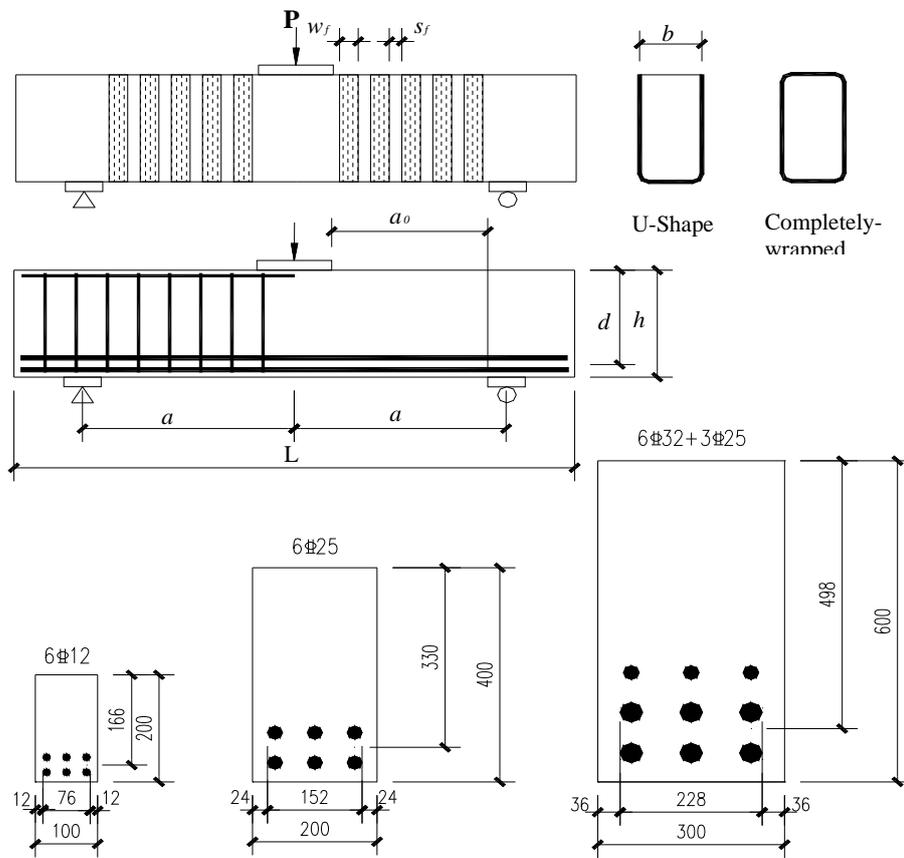
**Fig. 1.** Specimens configurations details
