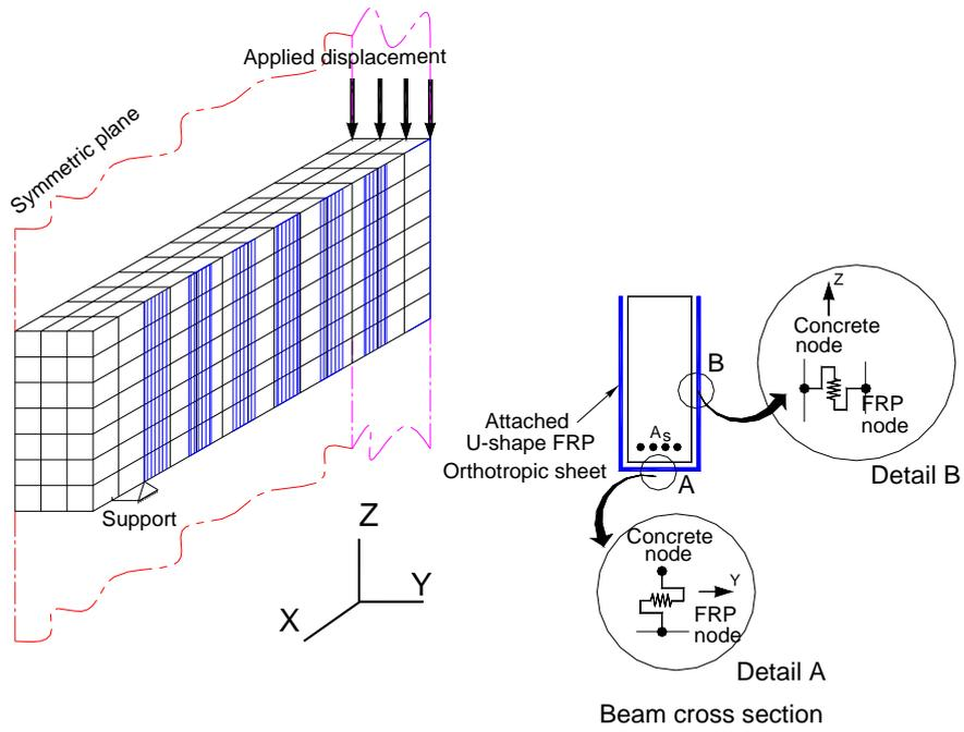
**Fig. 3.** Finite element model
