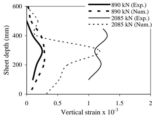
**Fig. 12.** Axial strain profiles along the CFRP depth for F3 bonded strip of specimen, W7
