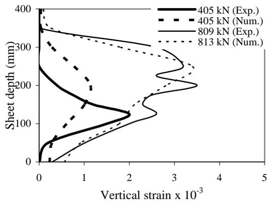
**Fig. 10.** Axial strain profiles along the CFRP depth for F3 bonded strip of specimens U5
