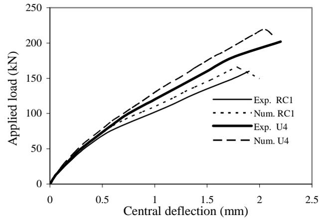
**Fig. 5.** Load–deflection relationships for the specimens of the first set
