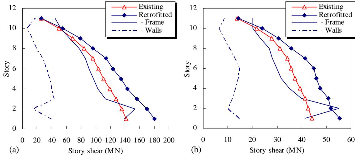
Figure 18 Story shear distributions along the height of the building and among different parts: (a) linear elastic and (b) nonlinear
