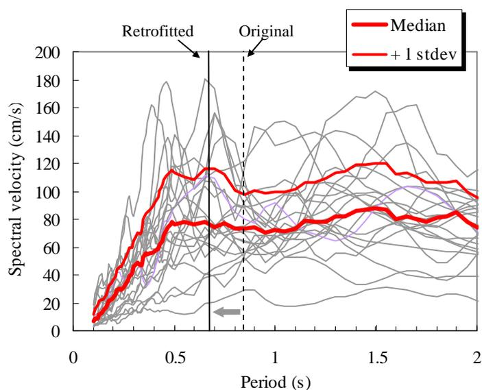
Figure 14 Spectral velocity of the 22 ground motion records normalized to  $PGV = 50 \text{ cm/s}$  (5%
