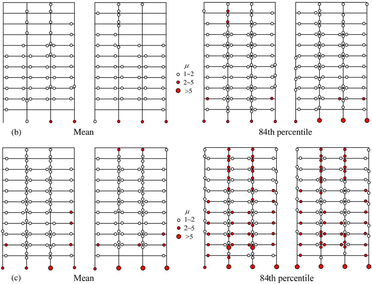
Figure 21 Ductility distributions of the outermost frame: (a) existing (original) structure; (b) retrofitted structure; and (c) retrofitted structure without dampers
