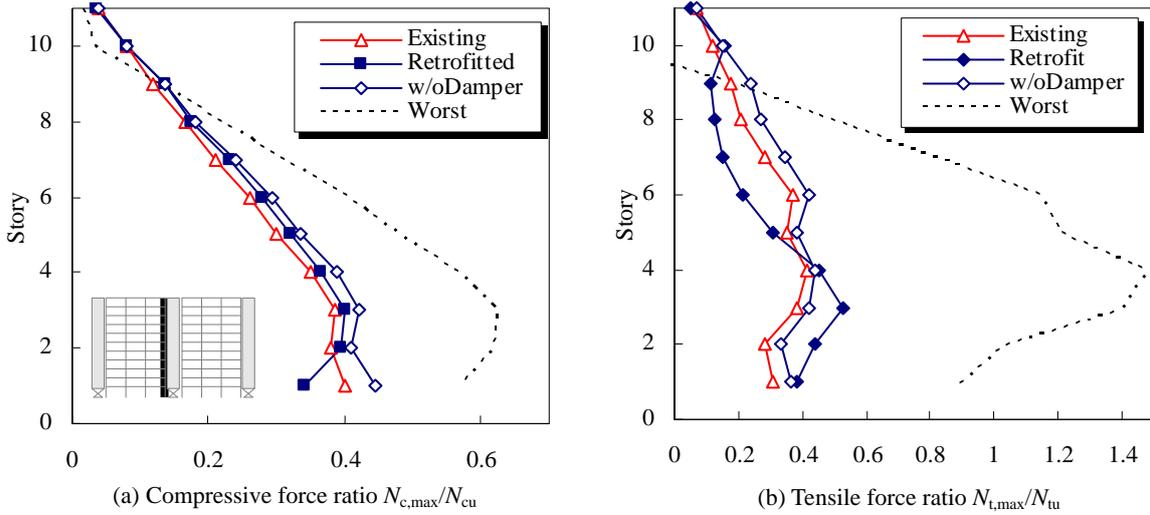
Figure 22 Median axial force ratios of columns
