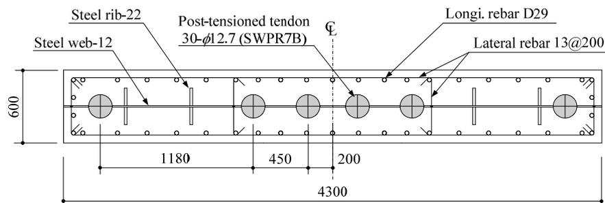
Figure 6 Cross section of post-tensioned wall
