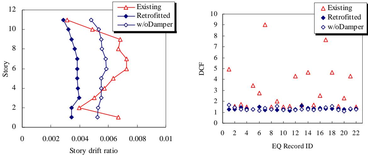
Figure 16 Median IDRs before and after retrofit
