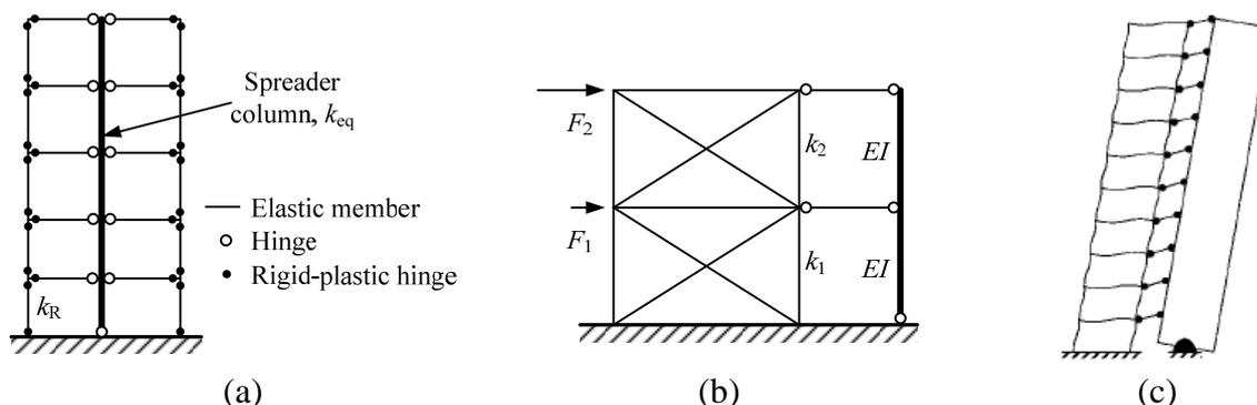
Figure 2 Structural models with pin-supported columns or walls: (a) spreader column by Akiyama (1984) [9]; (b) continuous column by MacRae et al. (2004) [11]; and (c) hinged wall by Alavi et al. (2004) [15]
