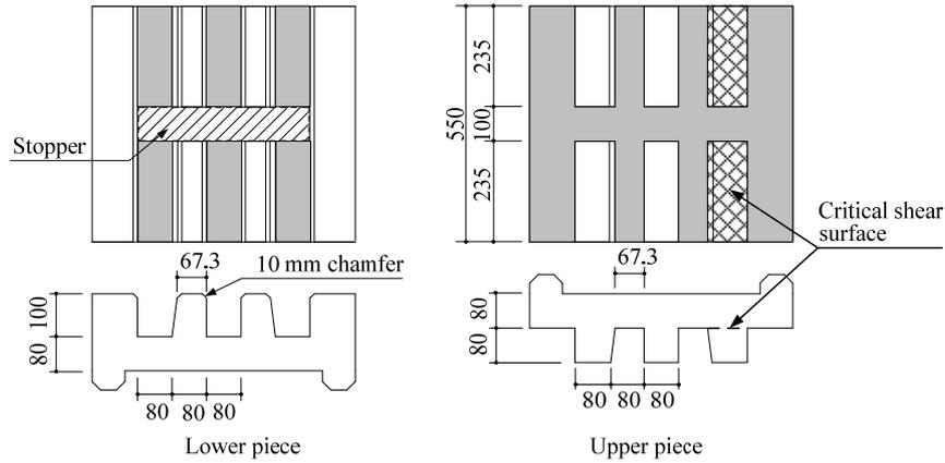
Figure 8 Details of pin bearing
