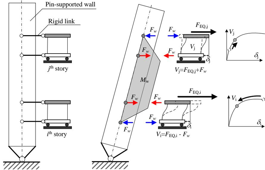
Figure 4 Mechanism of deformation pattern control by pin-supported walls
