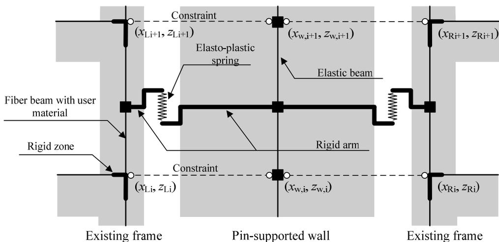
Figure 13 Modeling of pin-supported walls and steel dampers
