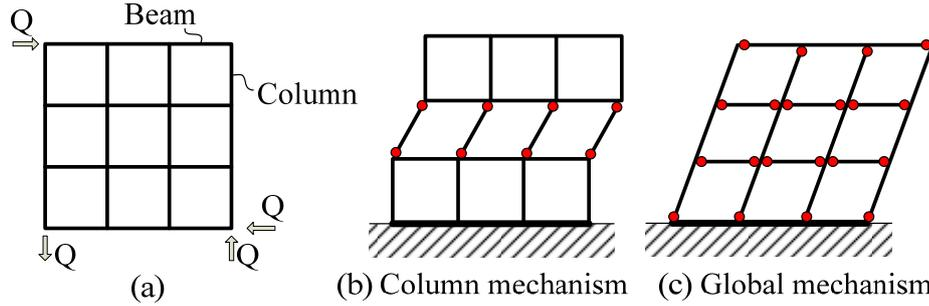
Figure 1 Possible plastic mechanisms of a moment-resisting frame under combined shear forces (Solid circles represent plastic hinges)
