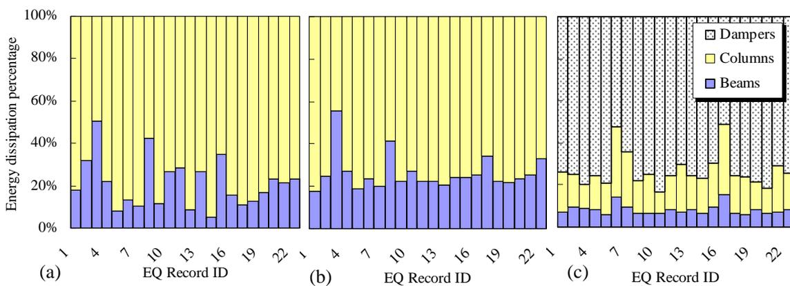
Figure 19 Distribution of energy dissipation among different types of components: (a) existing (original) structure; (b) retrofitted structure without dampers; and (c) retrofitted structure
