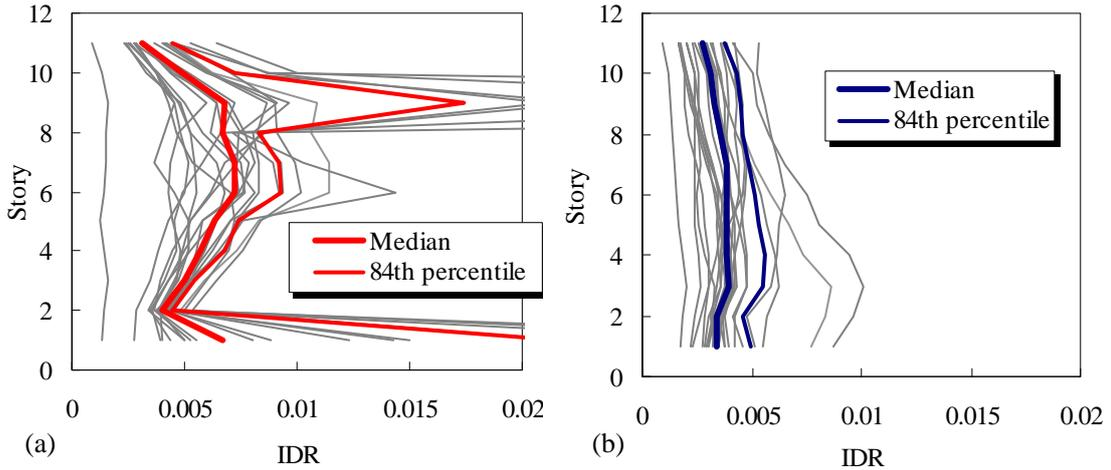
Figure 15 Story drift ratios of G3 Building before and after being retrofitted: (a) existing (original) structure and (b) retrofitted structure
