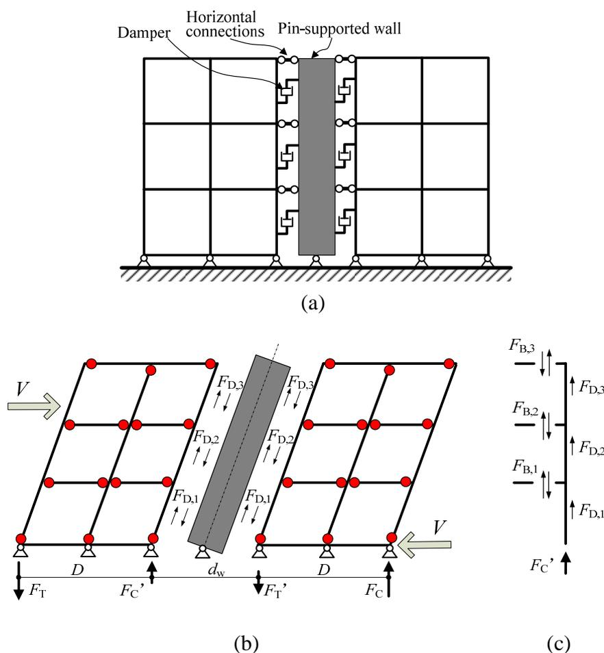
Figure 3 Pin-supported wall-frame system: (a) main components; (b) lateral resistance; and (c) vertical forces in the column connected with pin-supported wall
