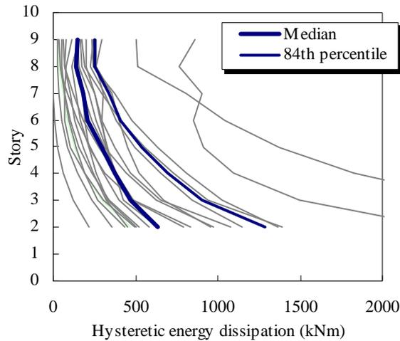
Figure 20 Distribution of hysteretic energy dissipated by steel dampers
