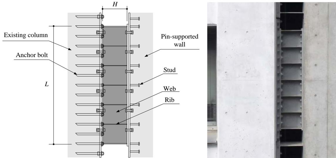
Figure 10 Completed steel damper with  $L = 1500$  mm
