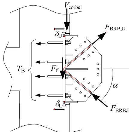
Figure 17. Force equilibrium of gusset plate during positive loading and measurement of gusset plate shear deformation.
