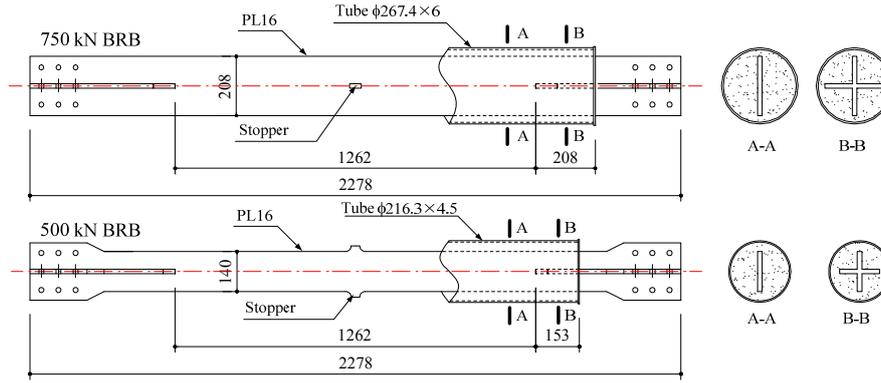
Figure 3. Buckling restrained braces.
