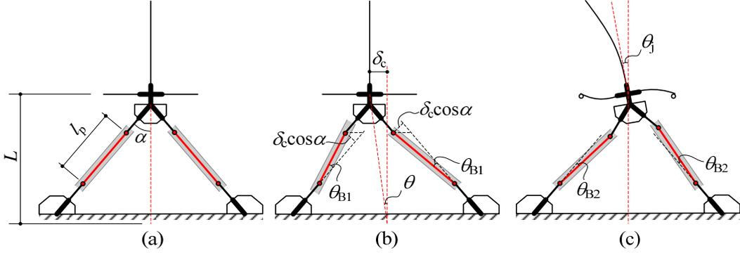
Figure 9. Mechanism of bending of BRBs: (a) undeformed shape, (b) deformation because of beam-to-column joint translation and (c) deformation because of beam-to-column joint rotation.
