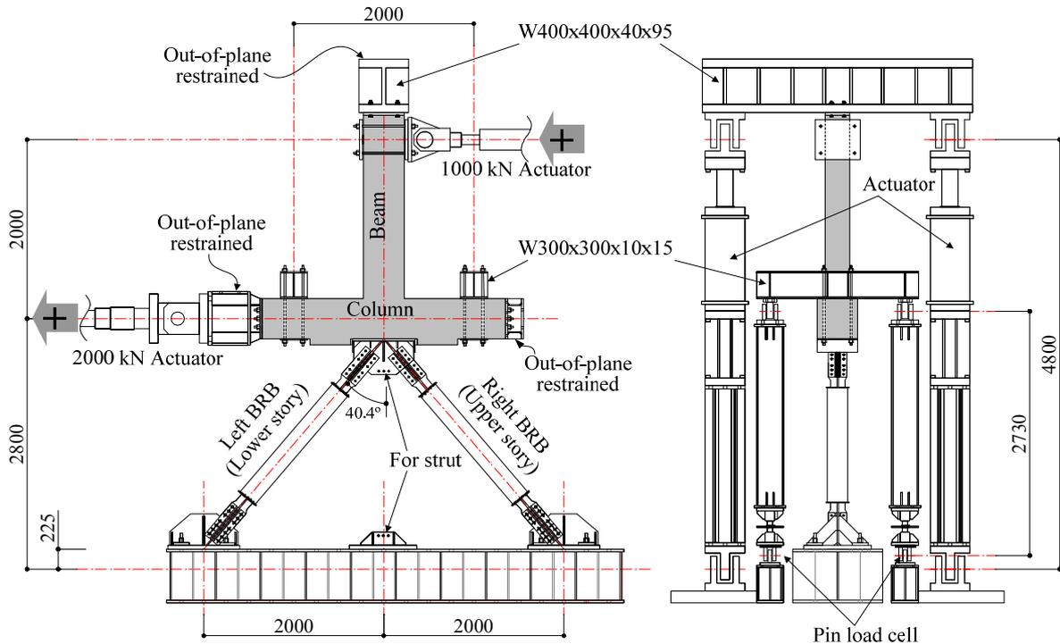
Figure 5. Test setup.
