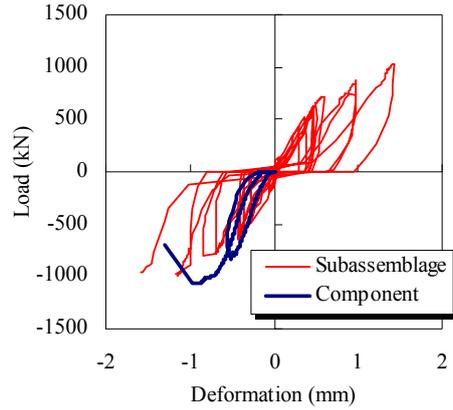
Figure 19. Corbel shear versus deformation relationship of Specimen No.1.
