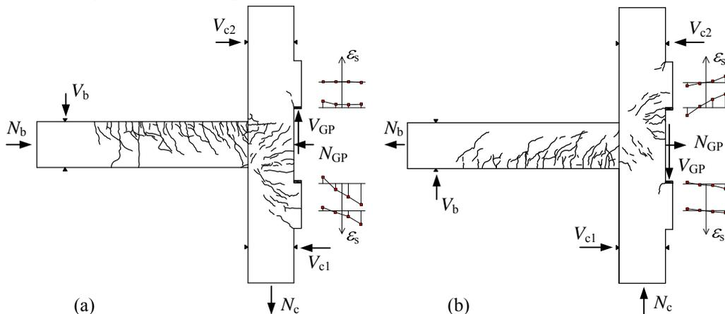
Figure 8. Cracks and strain of column longitudinal rebars of Specimen No.2 at: (a) +1/50 and (b) -1/50 story drift ratio.
