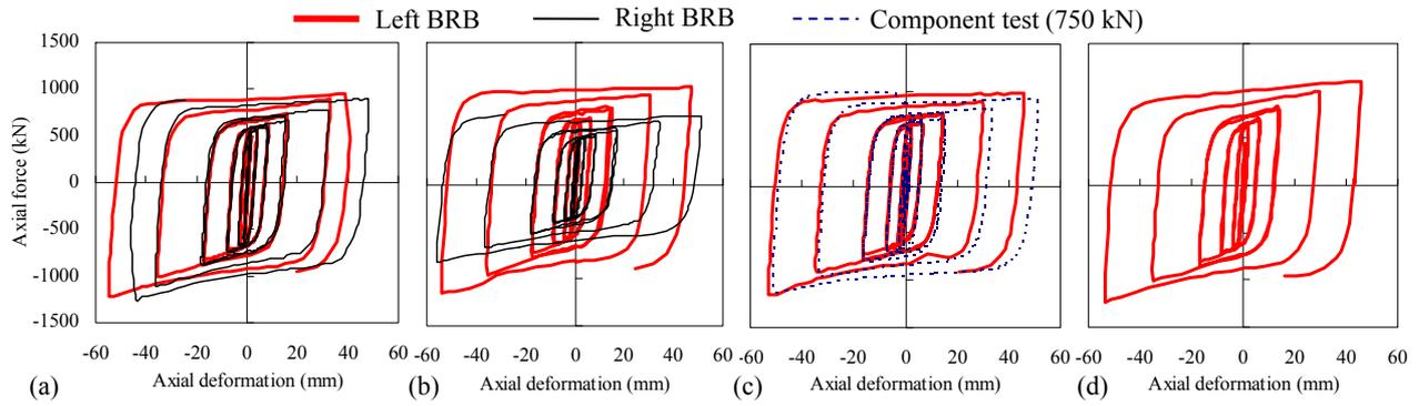
Figure 12. BRB hysteresis: (a) Specimen No.1, (b) No.2, (c) No.3 and (d) No.4.
