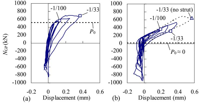
Figure 16. Relationship of force versus displacement of gusset plate normal to column surface: (a) Specimen No.3 and (b) No.4.
