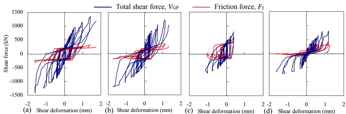
Figure 18. Shear resistance of gusset plate connection: (a) Specimen No.1, (b) No.2, (c) No.3 and (d) No.4.
