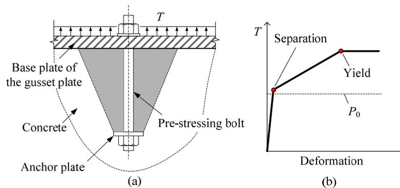
Figure 15. (a) Embedded pre-stressing bolt subjected to tension and (b) idealized tensile force-deformation relationship.
