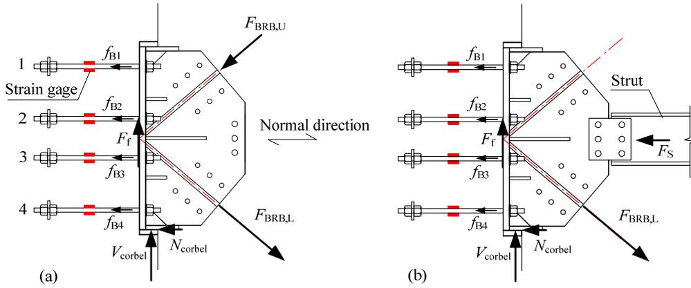
Figure 13. Force equilibrium of gusset plate during negative loading and measurement of bolt deformation: (a) Specimen No.3 and (b) No.4.
