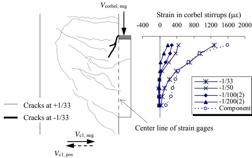
Figure 20. Cracks and stirrup strains of lower-story corbel of Specimen No.1.
