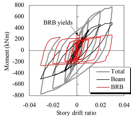
Figure 7. Moment resisting capacity of RC part in Specimen No.2.
