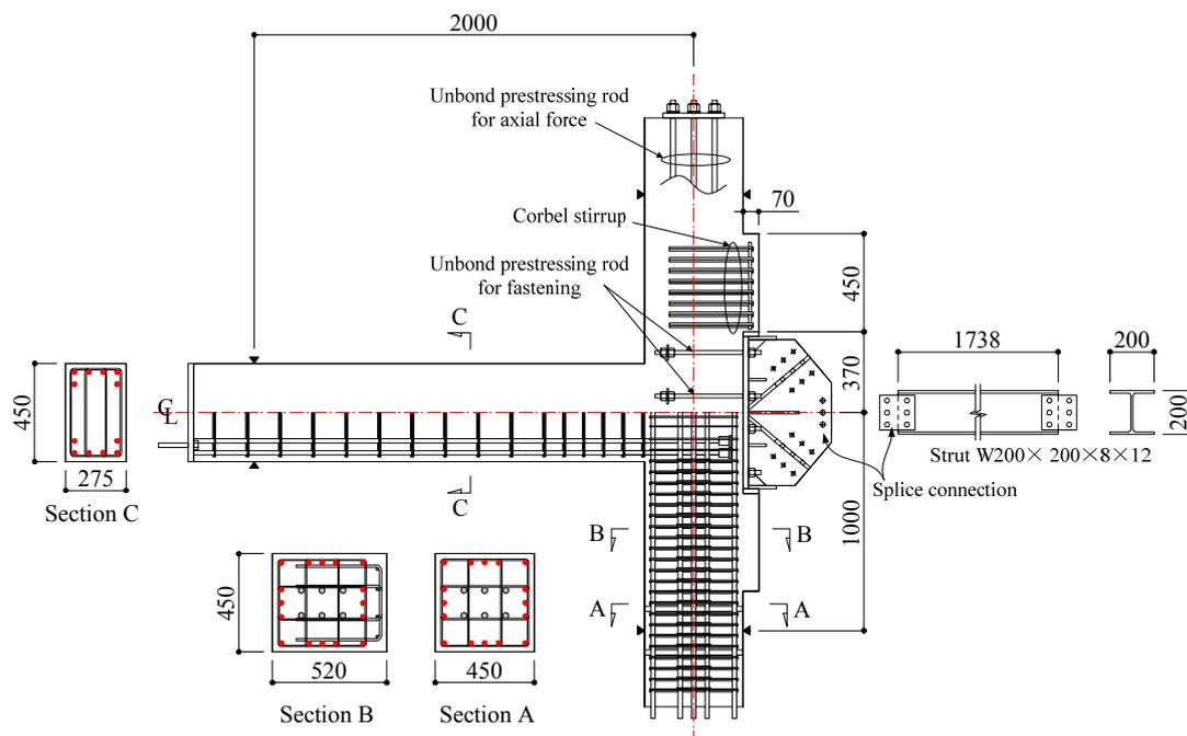
Figure 2. Reinforced concrete part of specimen with gusset plate installed and the strut.
