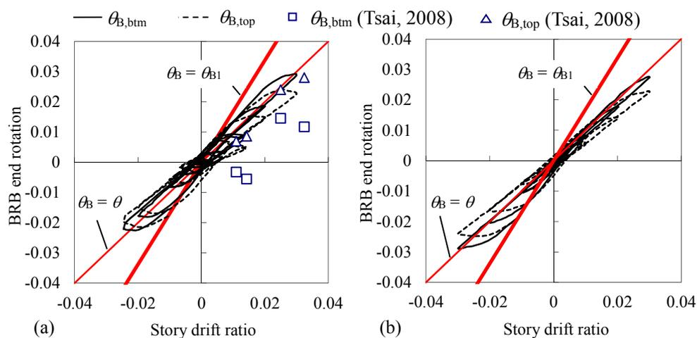
Figure 11. Measured end rotations of 750 kN left BRB (lower story) in (a) Specimen No.1 and (b) Specimen No.3.
