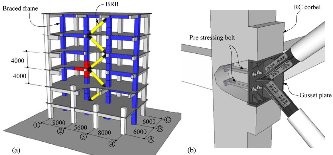
Figure 1. RC continuously buckling restrained braced frame: (a) structural layout and BRB configuration and (b) details of BRB connection.
