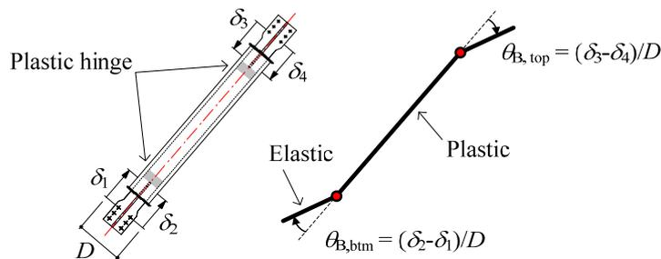
Figure 10. Measurement of BRB end rotation
