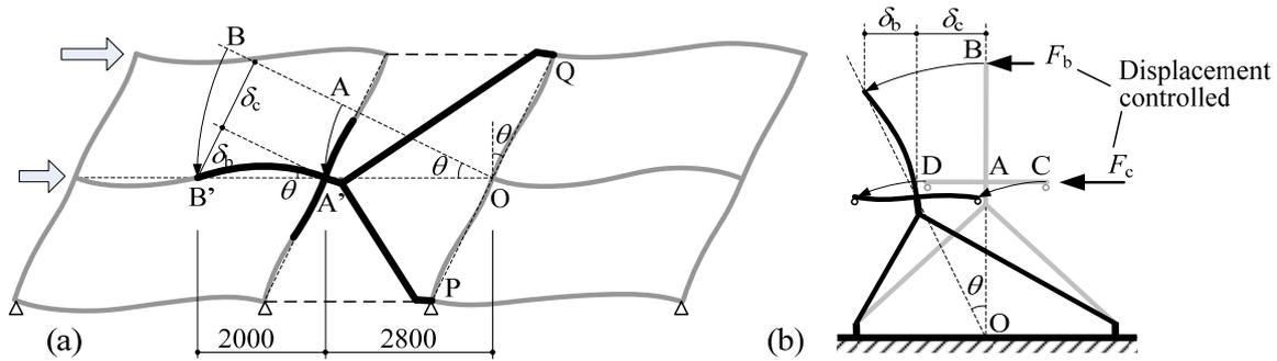
Figure 4. Deformed shape of subassembly.
