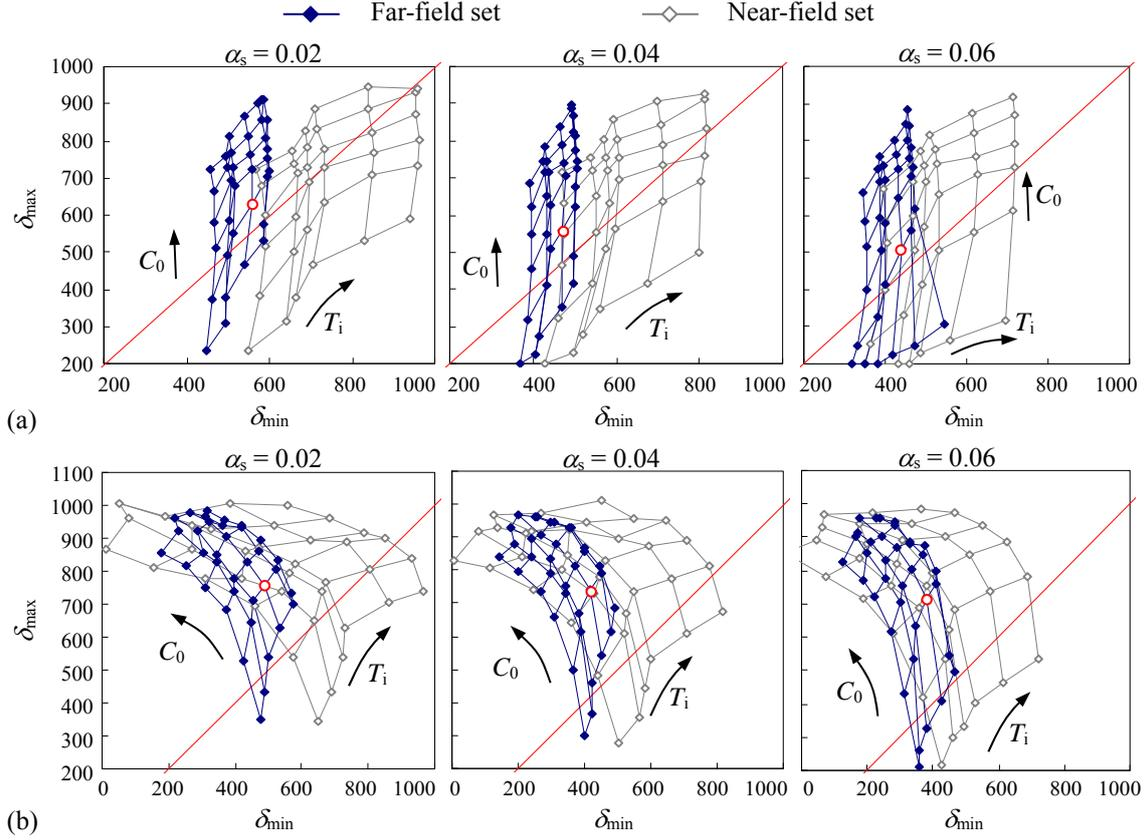
**Figure 9.** Gap graphs of base-isolated buildings with various amount of dampers subjected to either far-field or near-field motions ( $T_w = T_f$ ,  $nt_R = 200\text{mm}$ ): (a) non-ductile cases and (b) ductile cases.
