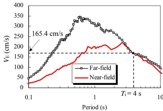
**Figure 4.** Median  $V_E$  spectra of the two sets scaled to  $V_E(4 \text{ s}) = 165.4 \text{ cm/s}$  (10% damping)
