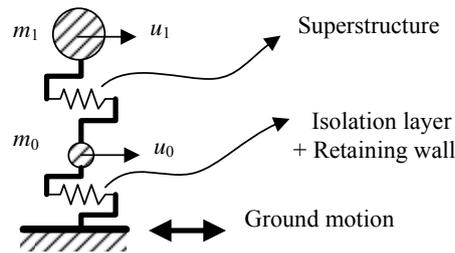
**Figure 1.** Lumped mass shear model
