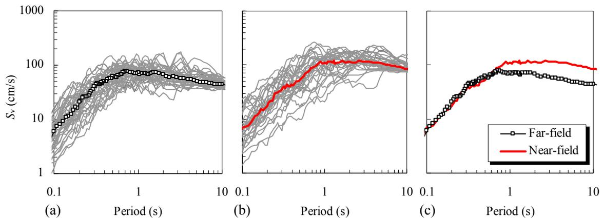
**Figure 3.** Spectral velocities of normalized ground motions (5% damping): (a) far-field set; (b) near-field set and (c) medians of the two sets
