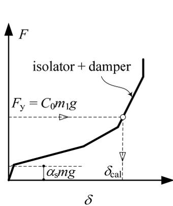
**Figure 12.** Model of calculating  $\delta_{\text{cal}}$  as an estimate of  $\delta_{\max}$
