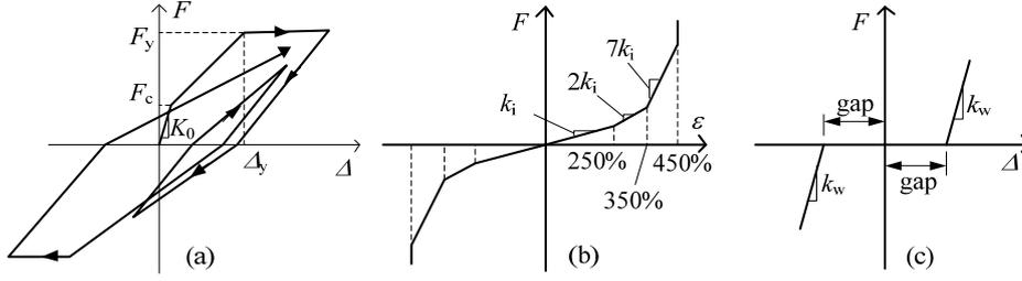
**Figure 2.** Hysteretic models for the base-isolated building: (a) superstructure, (b) natural rubber bearing and (c) retaining wall.
