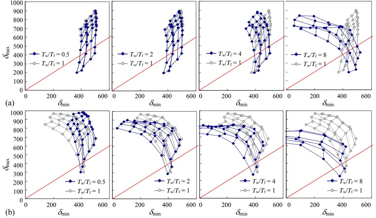
**Figure 10.** Influence of retaining walls stiffness on gap graphs ( $\alpha_s = 0.04$ ,  $nt_R = 200\text{mm}$ , Far-field set): (a) non-ductile limit-state and (b) ductile limit-state
