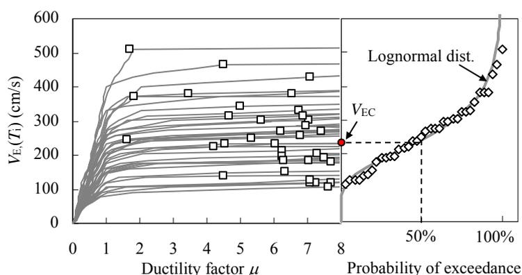
**Figure 5.** Median collapse capacity of ductile base-isolated building with  $C_0 = 0.15$ ,  $T_i = 4$  s,  $\alpha_s = 0.04$ ,  $T_w = T_f$ ,  $nt_R = 200$  mm and gap size = 500 mm under far-field set.
