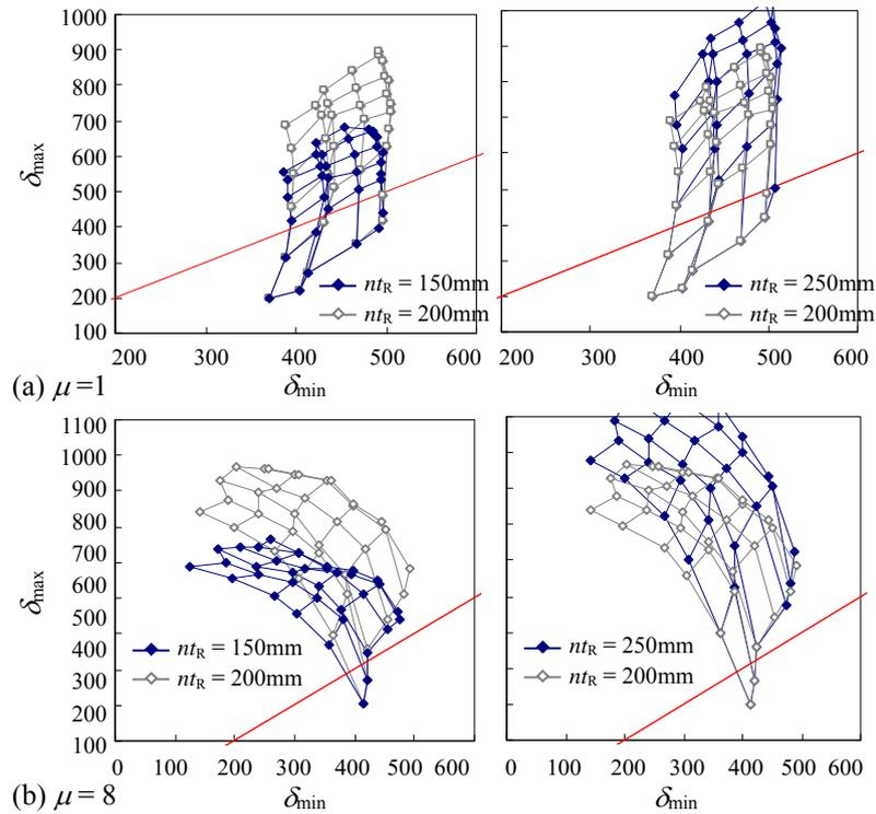
**Figure 11.** Influence of rubber thickness on gap graphs ( $\alpha_s = 0.04$ ,  $T_w = T_i$ , Far-field set): (a) non-ductile limit-state ( $\mu = 1$ ) and (b) ductile limit-state ( $\mu = 8$ )
