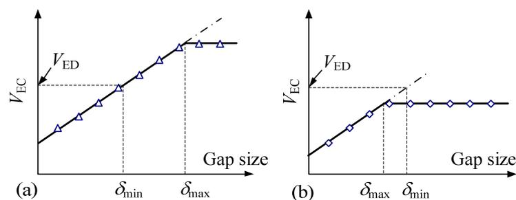
**Figure 7.** Characteristic gap sizes of base-isolated building: (a) when  $\delta_{\min}$  is less than  $\delta_{\max}$  and (b) when  $\delta_{\min}$  is greater than  $\delta_{\max}$
