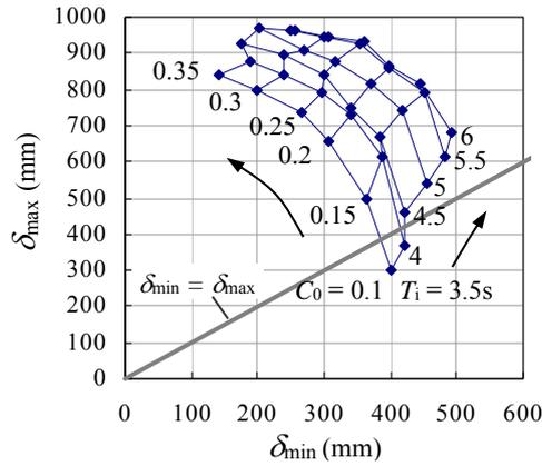
**Figure 8.** Gap graph of ductile base-isolated buildings with  $\alpha_s = 0.04$ ,  $T_w = T_f$  under far-field set
