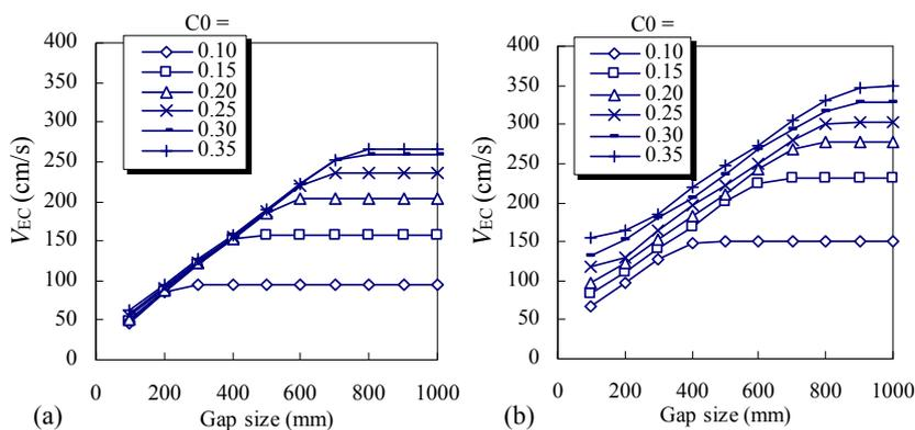
**Figure 6.** Influence of gap size on limit-state capacity ( $T_i = 4$  s,  $\alpha_s = 0.04$ ,  $T_w = T_i$ ,  $nt_R = 200$  mm, far-field set): (a) non-ductile cases and (b) ductile cases
