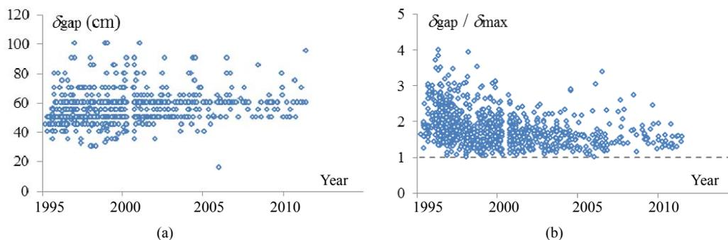
**Figure 1.** Statistics of isolation gap width of 979 seismically base-isolated buildings in Japan: (a) isolation gap width,  $\delta_{\text{gap}}$  and (b) ratio of isolation gap width to maximum displacement,  $\delta_{\text{gap}}/\delta_{\text{max}}$ .
