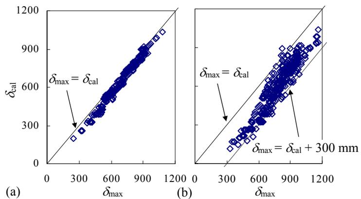
**Figure 13.** Relationship of  $\delta_{\max}$  versus  $\delta_{\text{cal}}$ : (a) non-ductile limit-state and (b) ductile limit-state
