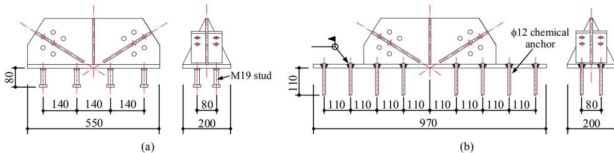
Figure 2.2 Connection details for gusset plates on beams: (a) embedded shear studs for new construction applications; (b) post-installed anchors for seismic retrofit applications.
