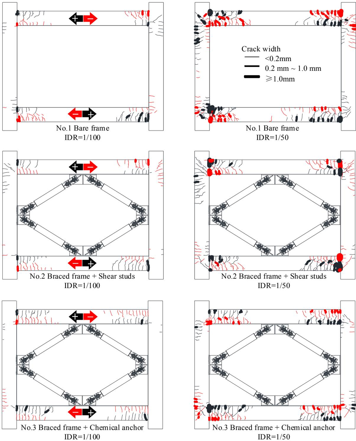
Figure 4.2 Cracks on RC frames
