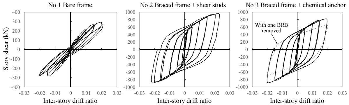
Figure 4.1 Force-displacement relationship of specimens
