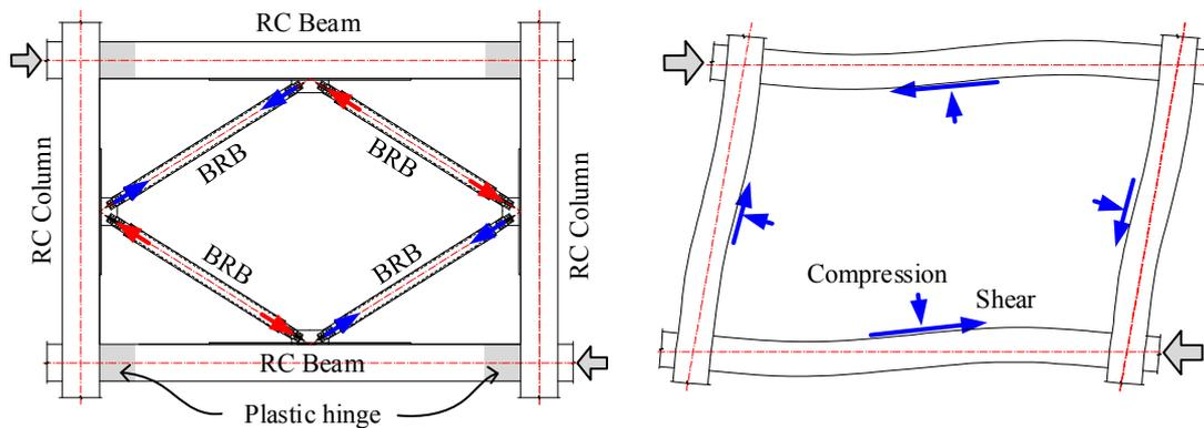
Figure 1.1 Reinforced concrete frames braced by BRBs in double-K configuration
