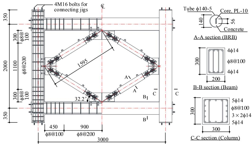
Figure 2.1 Specimen geometry and reinforcement
