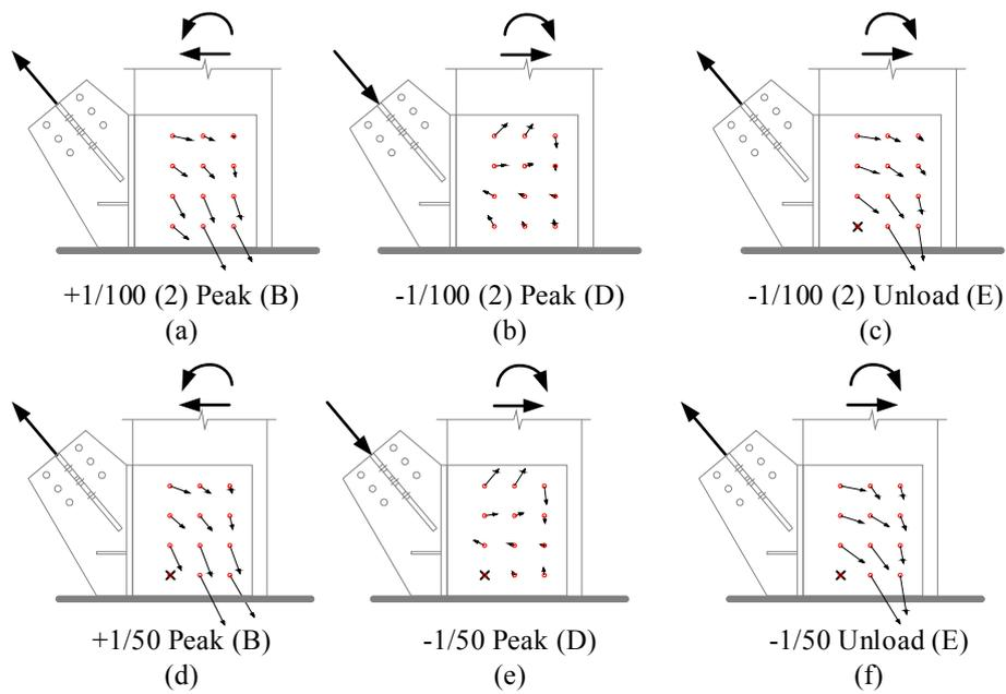
FIG. 16. Direction and magnitude of curvature at stud ends of Specimen No.5 (EB+DC).
