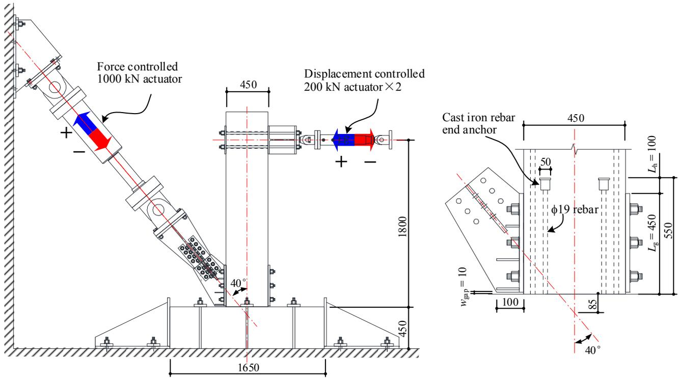
Fig. 4. Test setup and dimensions (length unit: mm).
