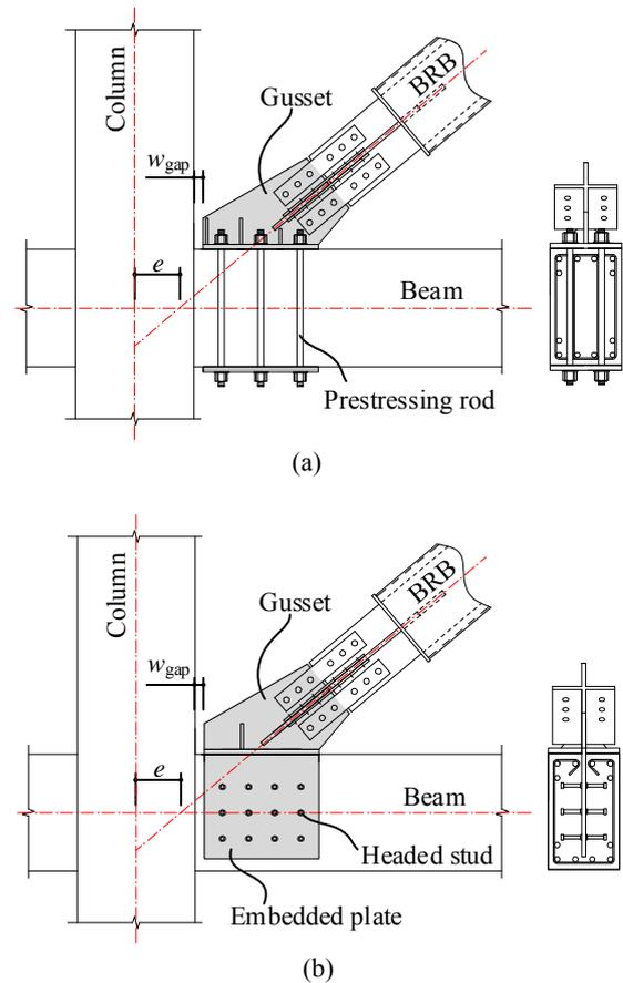
Fig. 1. Proposed unconstrained gusset connections: (a) post-tensioned type (PT) and (b) embedded plate type (EB).
