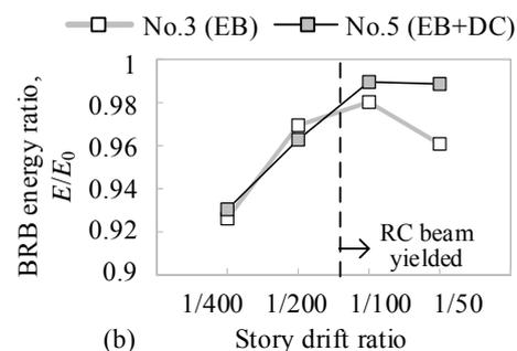
FIG. 11. BRB energy ratio: (a) PT specimens and (b) EB specimens.
