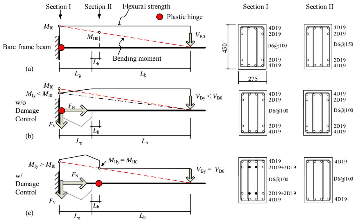
Fig. 2. Control of beam plastic hinge location: (a) Bare beam, (b) braced beam without damage control and (c) braced beam with damage control.
