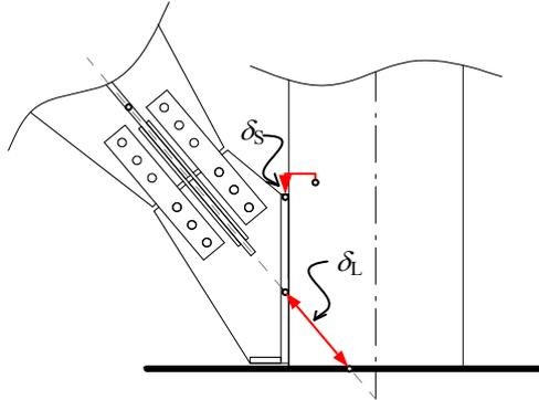
FIG. 8. Measurement for deformation loss at gusset connection.
