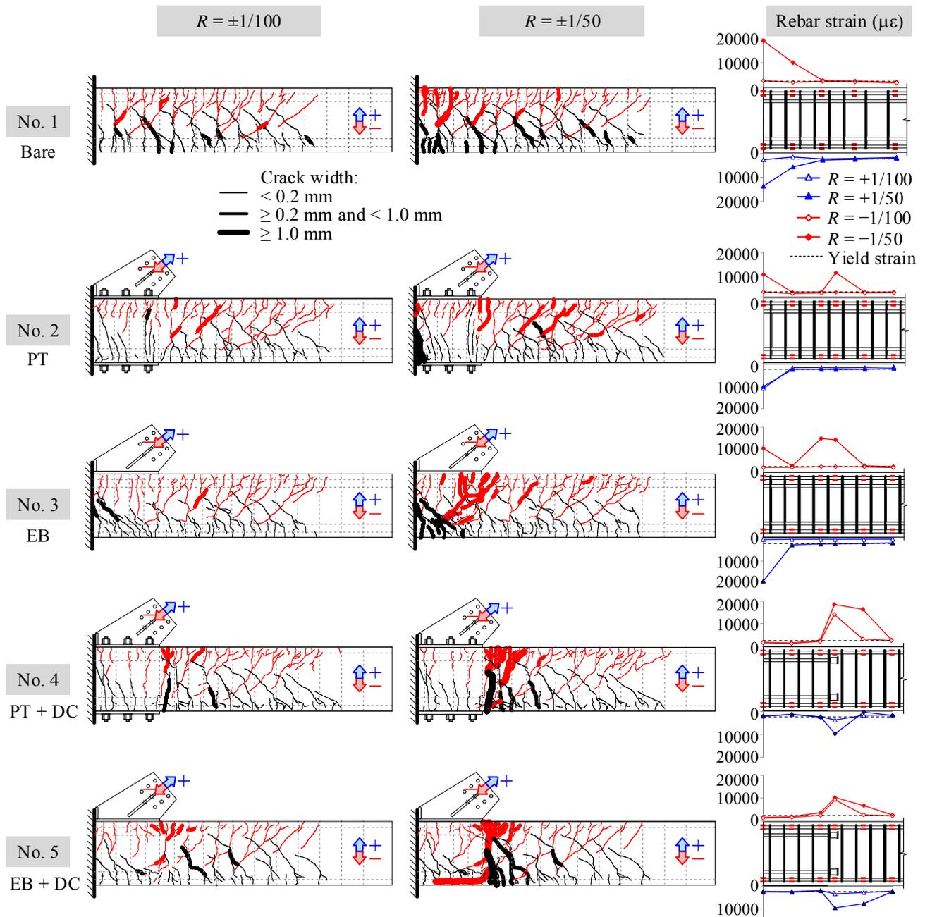
FIG. 7. Damage to RC beams.
