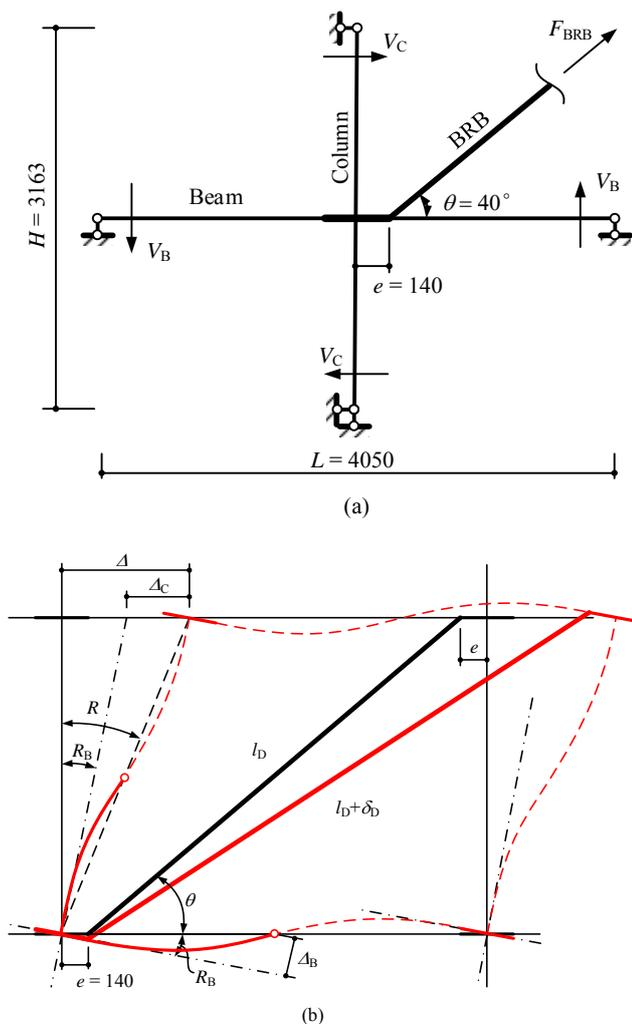
Fig. 3. Subassembly of buckling restrained braced frame: (a) un-deformed and (b) deformed configuration.
