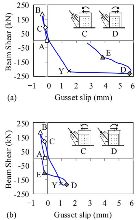
FIG. 12. Gusset slip during 1/50 load cycle: (a) Specimen No.3 and (b) No.5.
