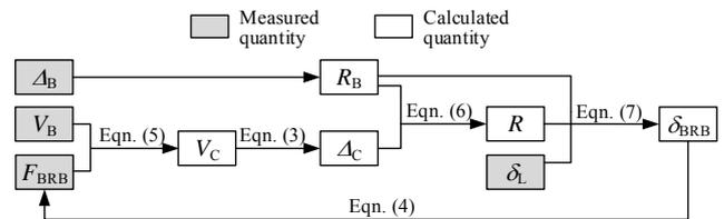
Fig. 5. Flowchart of load control process in a single load increment.
