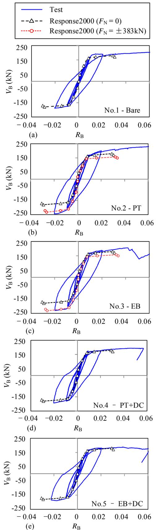
FIG. 6. Shear force and chord rotation of RC beam: (a) Specimen No.1; (b) No.2; (c) No.3; (d) No.4 and (e) No.5.
