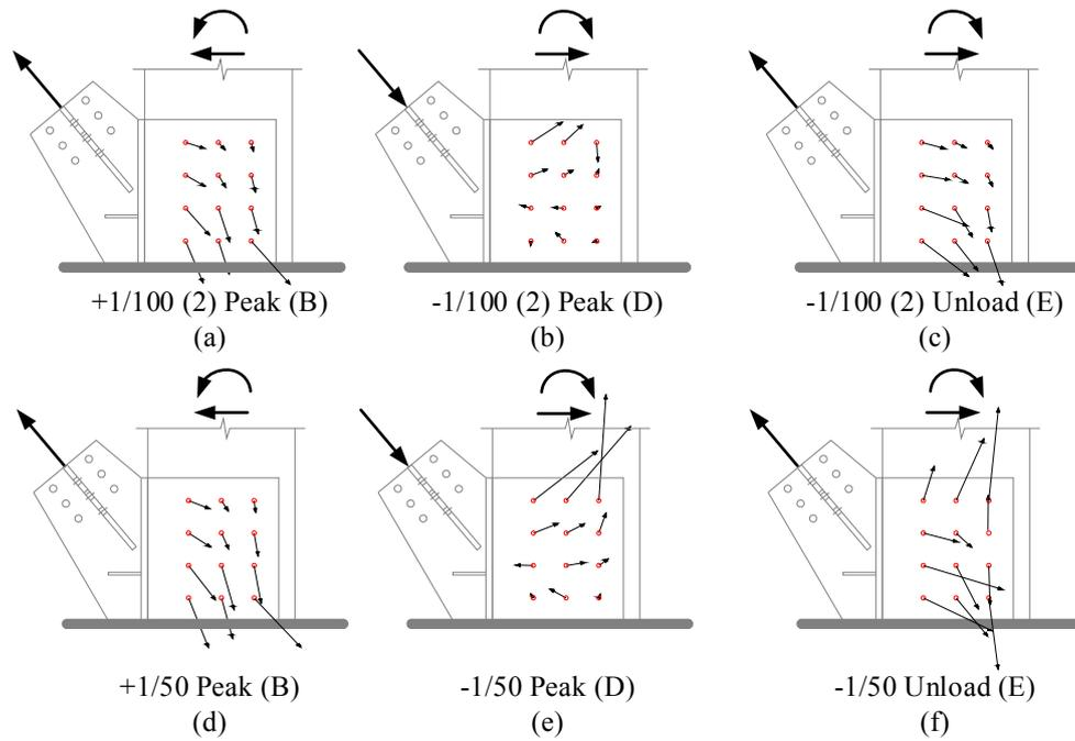
FIG. 15. Direction and magnitude of curvature at stud ends of Specimen No.3 (EB).
