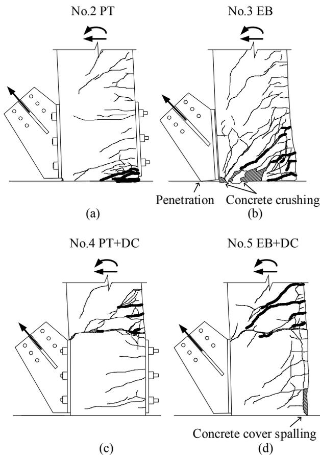
FIG. 13. Deformed shape of RC beam end at 1/20 story drift of (a) Specimen No.2, (b) No.3, (c) No.4 and (d) No.5.
