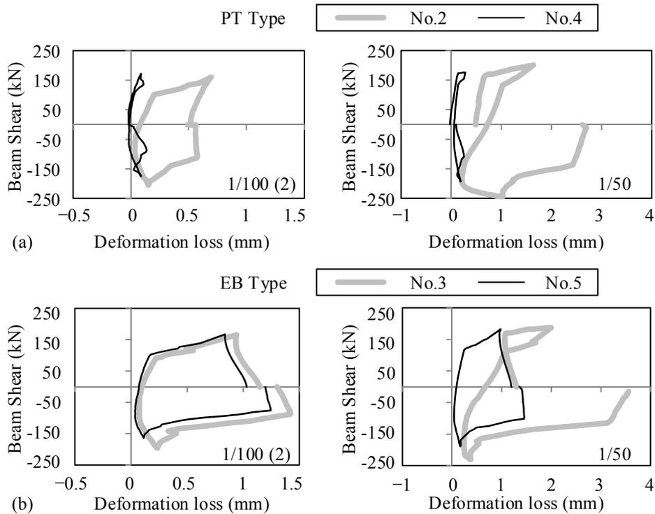
FIG. 10. Deformation loss at gusset connection: (a) Specimen No.2 and No.4, PT type and (b) No.3 and No.5, EB type connection.
