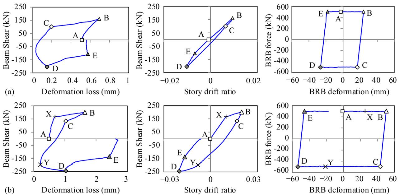
FIG. 9. Development of deformation loss at gusset connection of Specimen No.2, PT: (a) 1/100 load cycle and (b) 1/50 load cycle.
