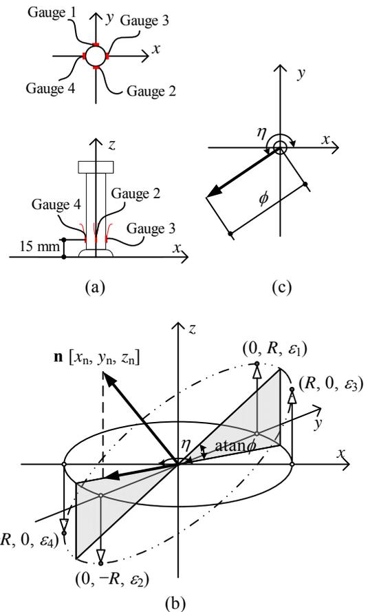
FIG. 14. Calculation of curvature at end of stud from strain readings.
