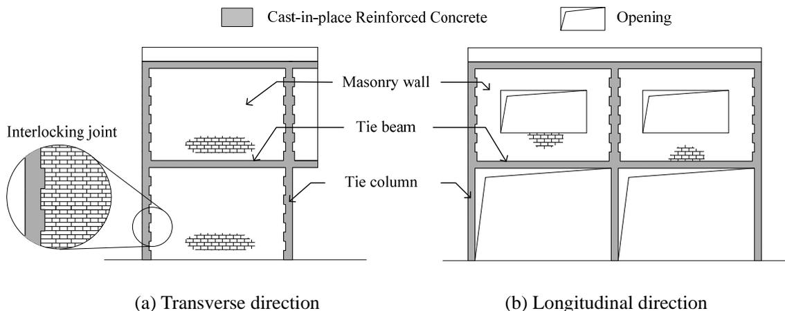
**Figure 3.** Structural configuration of confined masonry house
