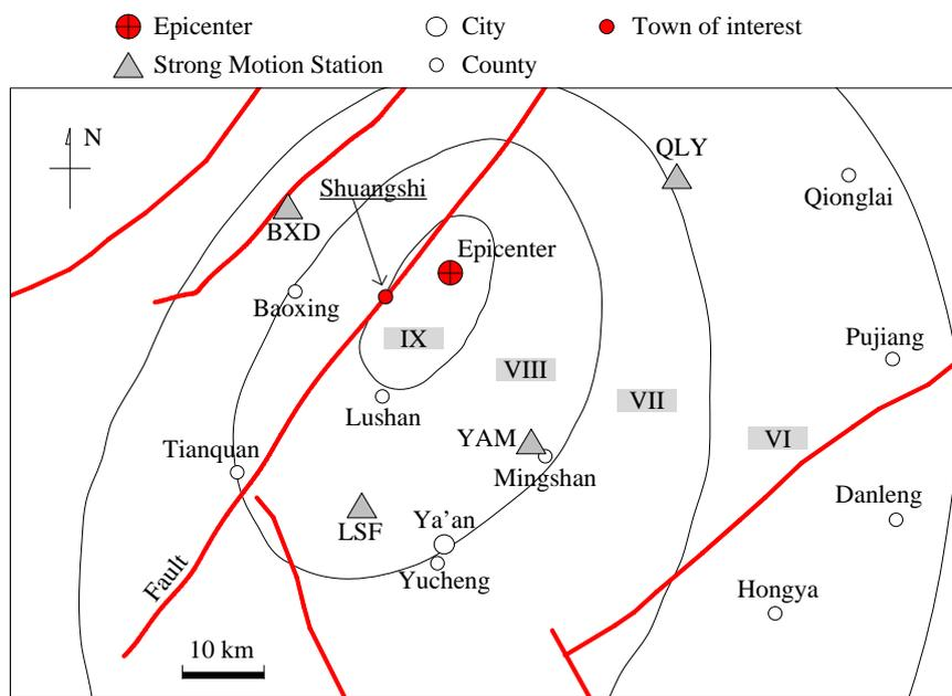
Figure 1. Intensities, faults and strong motions stations in near field area of Lushan earthquake.
