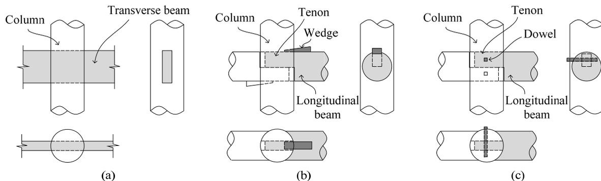
**Figure 5.** Typical beam-to-column joints in Chuandou timber houses: (a) transverse beam-to-column penetration joint; (b) longitudinal beam-to-column mortise-and-tenon joint with wedge and (c) longitudinal beam-to-column mortise-and-tenon joint with dowel.
