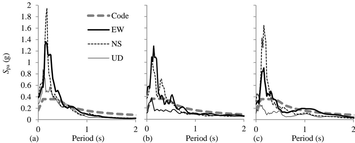
**Figure 2.** Pseudo acceleration spectrum of ground motion records at (a) LSF station; (b) YAM station and (c) QLY station.
