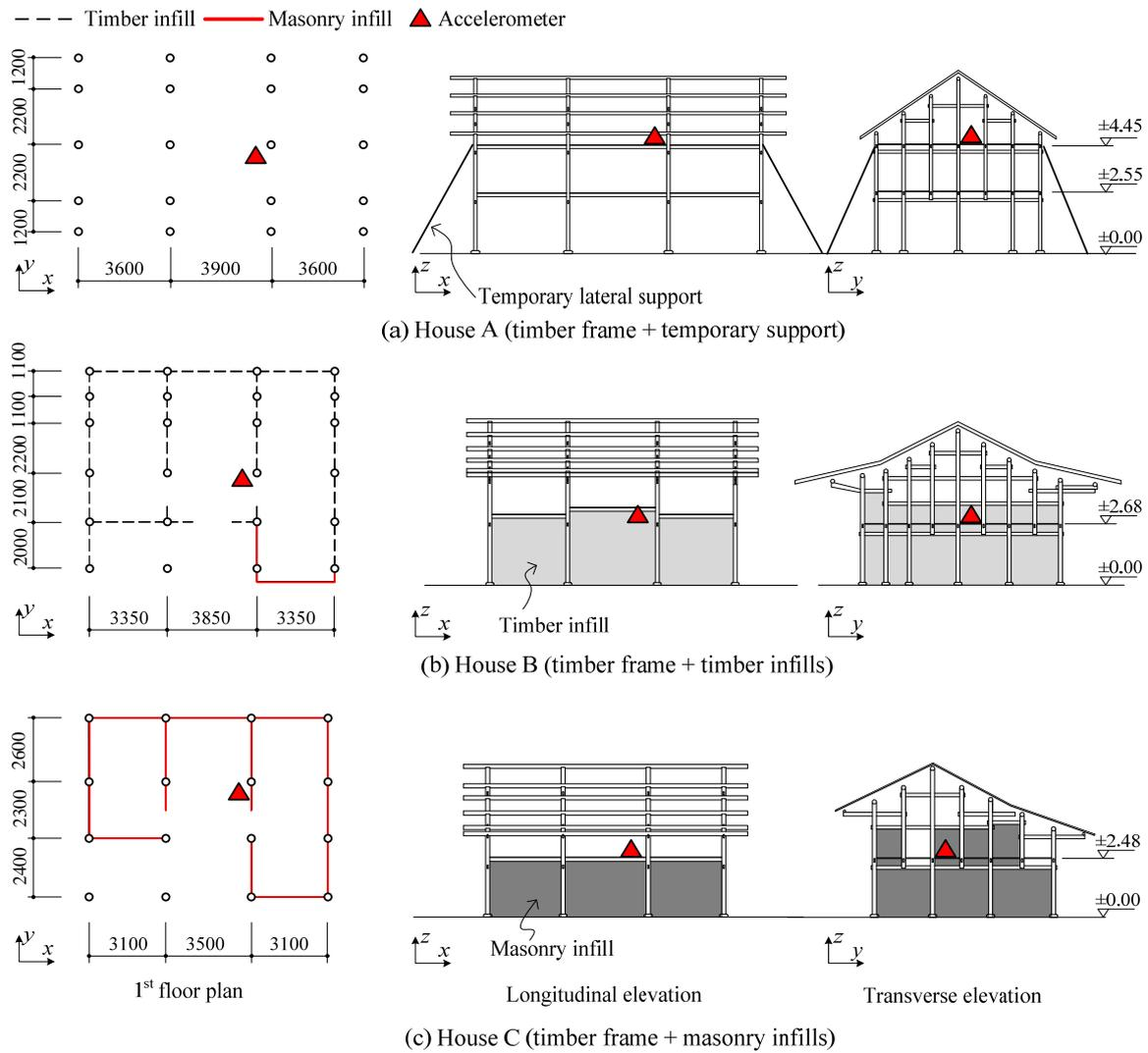
**Figure 6.** Structural layout and locations of accelerometers of (a) House A; (b) House B and (c) House C.
