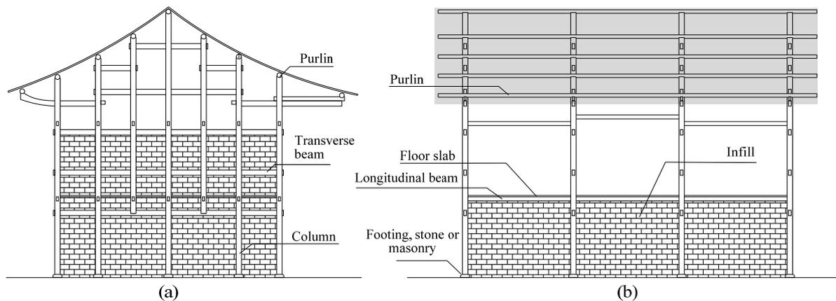
**Figure 4.** Structural configuration of Chuandou timber houses with infills: (a) transverse elevation and (b) longitudinal elevation.
