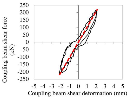
Fig. 6: Determination of initial stiffness of specimen
