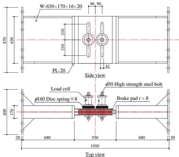
Fig. 2: Specimen of steel coupling beam with friction damper.
