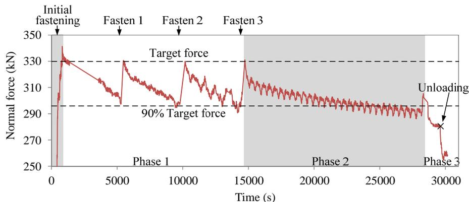
Fig. 9: Variation of normal force on the frictional interface.
