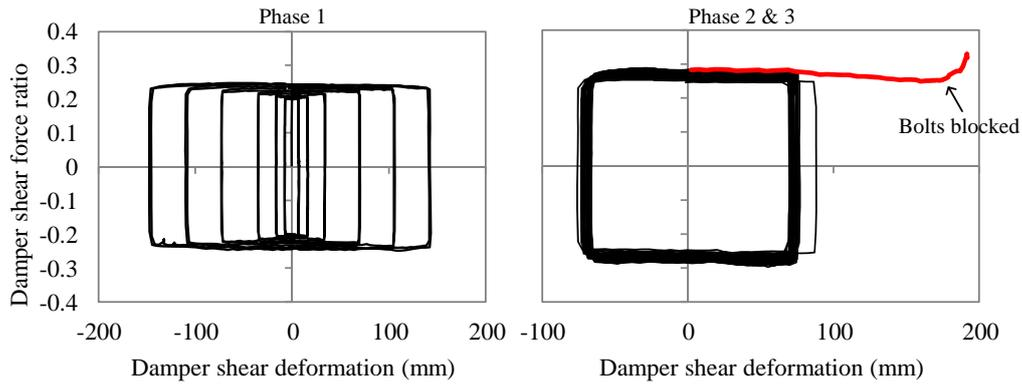
Fig. 8: Load-deformation hysteresis of friction damper.
