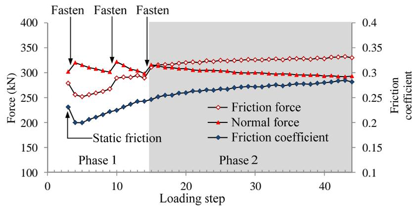
Fig. 10: Variation of friction coefficient of the brake pad-to-steel interface.
