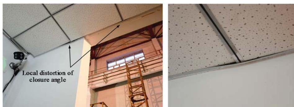
Fig.17 Damage to perimeter runners in shake table tests (run 5)
