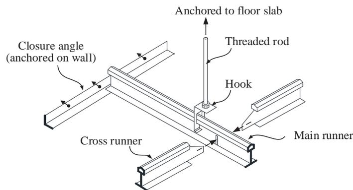
Fig.1 Basic components of ceiling grids
