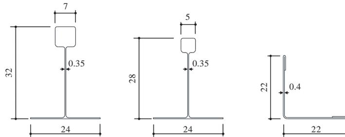
Fig.12 Cross section dimensions of grid components
