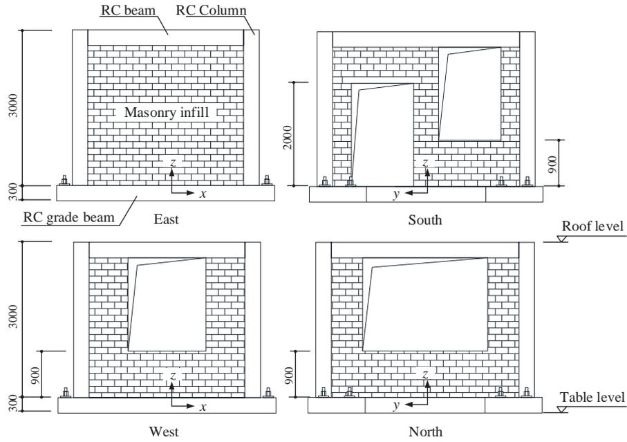
Fig. 9 Elevations of RC frame
