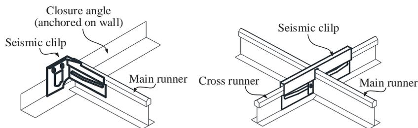
Fig.2 Seismic clips for suspended ceiling grids (reproduced based on CIBSDR, 2012)
