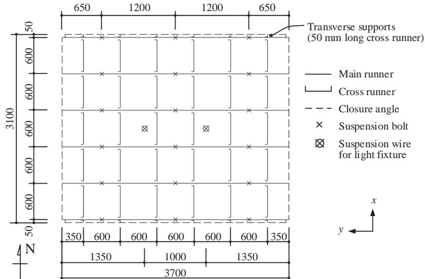
Fig.11 Suspended ceiling layout
