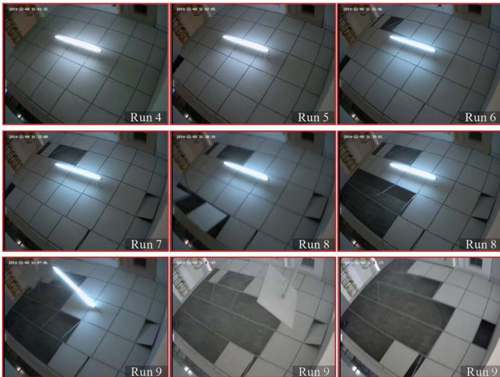
Fig.15 Falling process of ceiling panels
