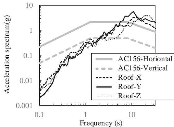
Fig.14 Acceleration spectra of roof motions in run 5 compared with required response spectra in AC156 (2012)
