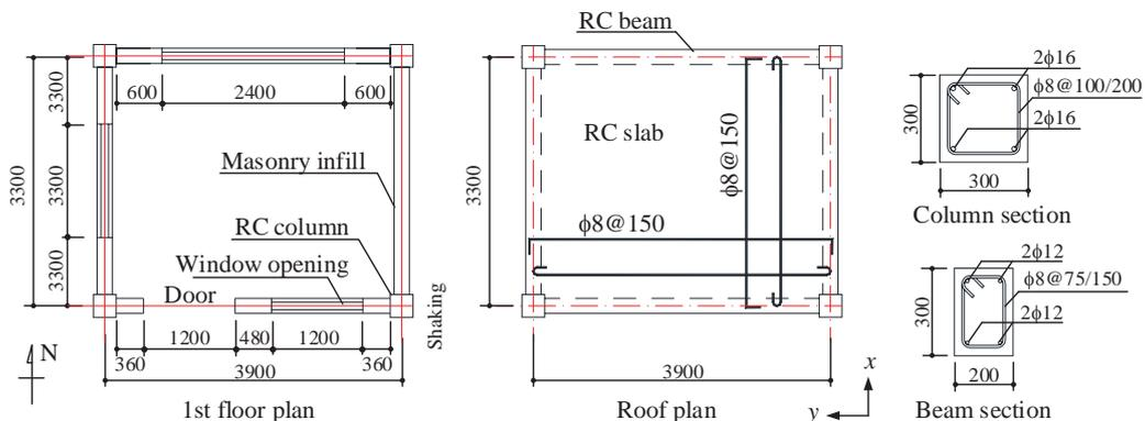
Fig. 8 Structural layout of RC frame for loading
