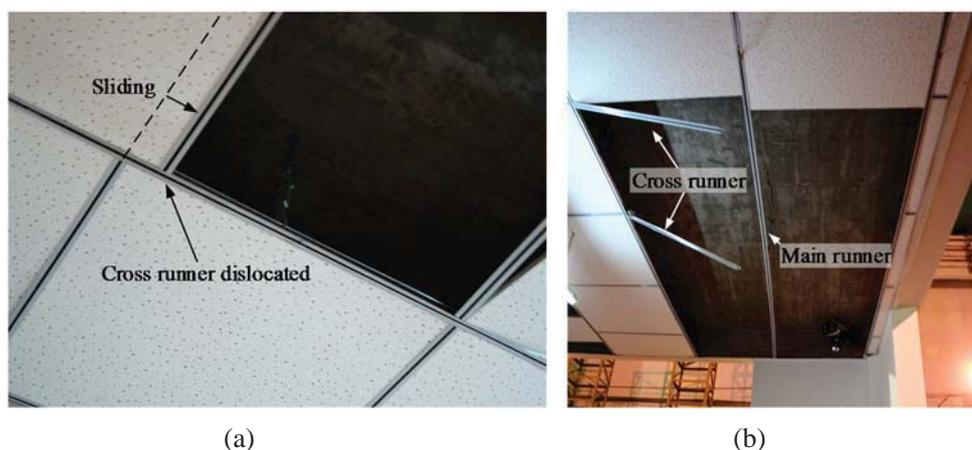
Fig.16 Damage to cross tees in shake table tests (run 7 and 8)
