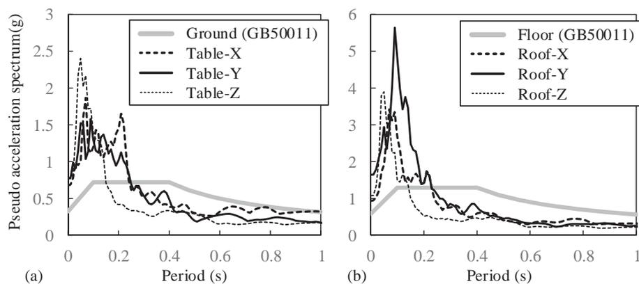
Fig.18 Acceleration spectra of table and roof motions compared with design spectra for Lushan in Chinese seismic code (run 5)
