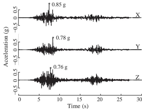
Fig.13 Time history of earthquake motion for input (run 5)
