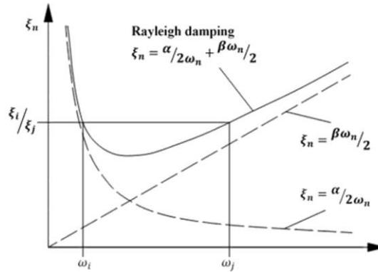
Fig.1 Rayleigh damping model
