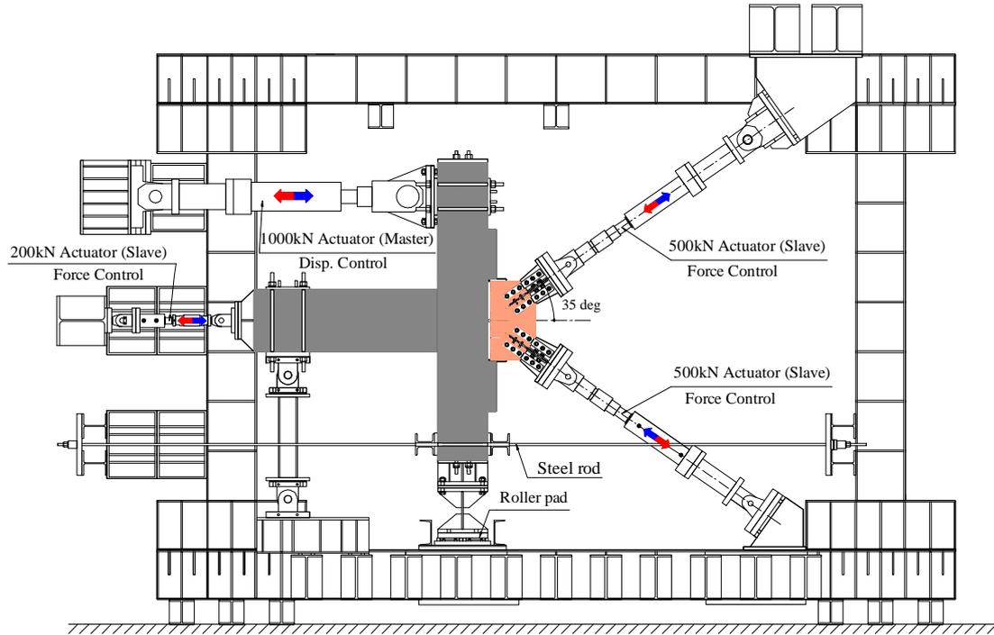
Figure 3. Side view of the experimental setup
