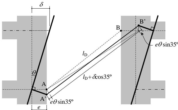
Figure 4. Change in the work point-to-work point brace length
