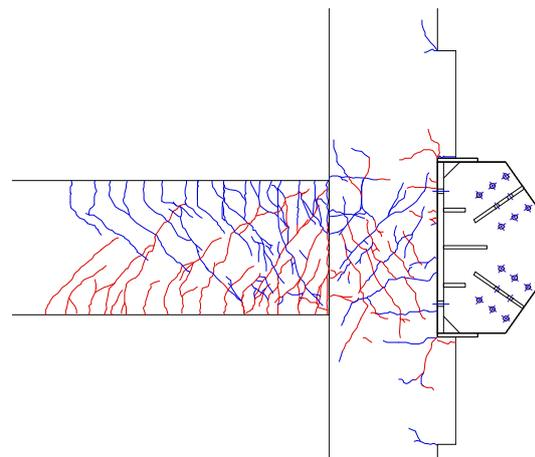
Figure 7. Cracking pattern of Specimen No.3-Weak corbel at 1/33 story drift ratio
