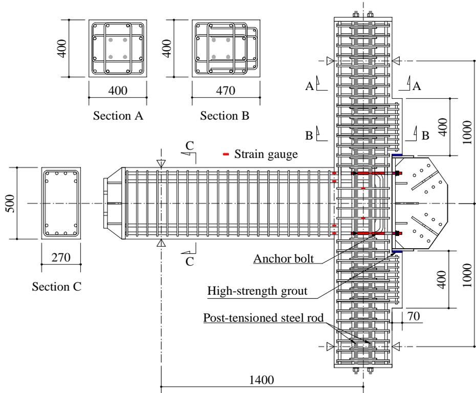
Figure 2. Dimensions and reinforcement of Specimen No.1 (Standard)
