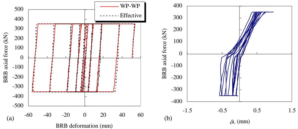
Figure 8. Deformation of the lower BRB in Specimen No.3-Weak corbel: a) BRB global deformation; b) Deformation loss in the connections
