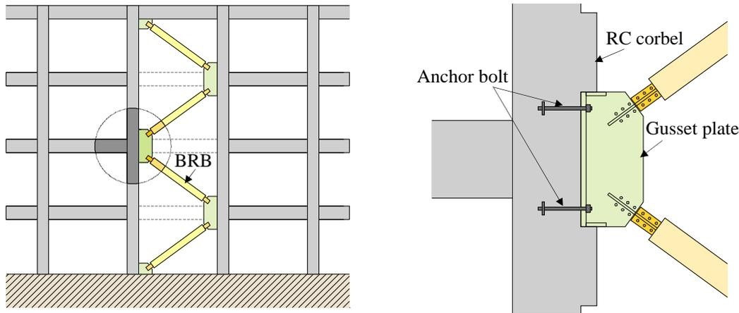
Figure 1. RC continuously braced frame: a) BRB arrangement b) BRB connection
