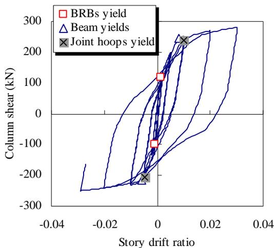
Figure 6. Story drift ratio-column shear relation of Specimen No.3-Weak corbel
