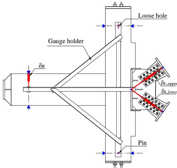
Figure 5. The gauge holder and locations of displacement transducers
