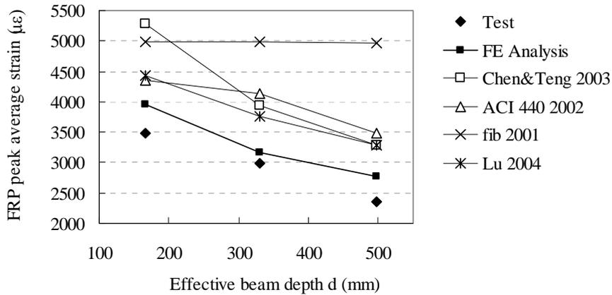
Figure 9 The peak average strains of FRP sheets
