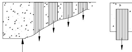
(a) FRP externally bonded on the web in shear      (b) Direct-pull test
