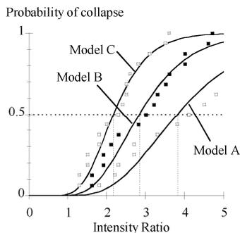
Figure 4 An example of fragility curves of isolated structure
