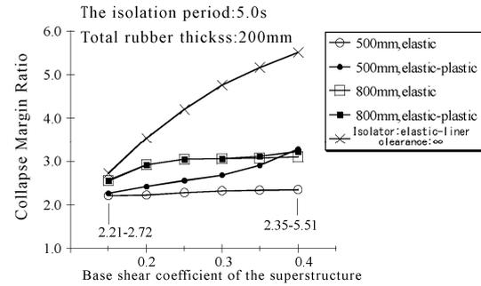
Figure 7 Influence of retaining wall behavior, superstructure strength and clearance size
