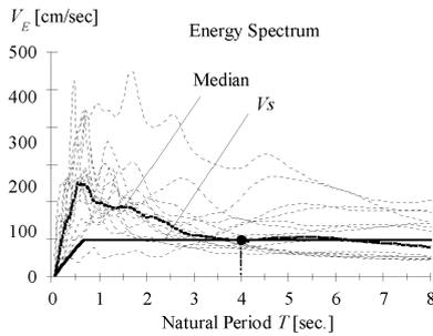
Figure 2 Equivalent velocity spectrum of normalized records when  $IR=1.0$
