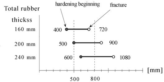
Figure 5 Characteristic deformations of the isolator compared with the size of clearance
