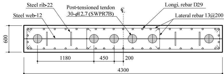
Figure 5. Cross section of post-tensioned wall.
