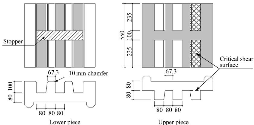
Figure 7. Details of pin bearing.
