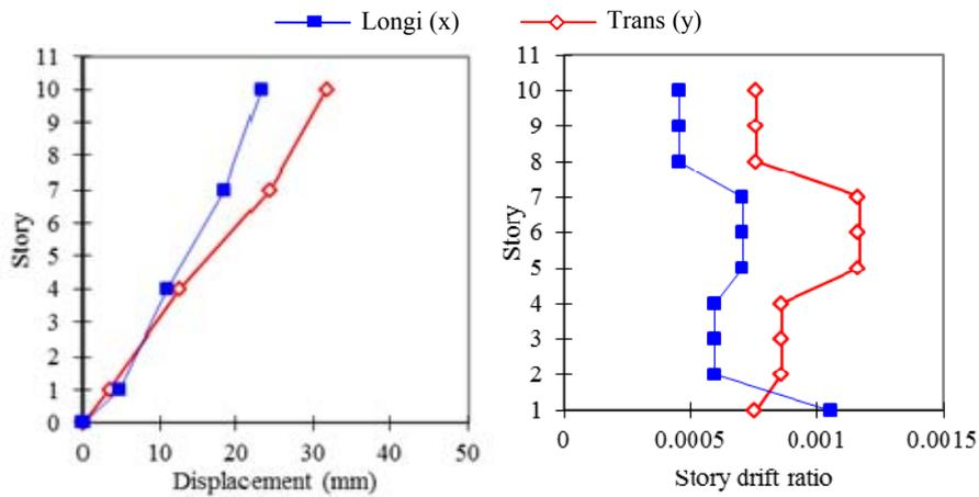
Figure 11. Recorded peak motions of G3 Building: (a) lateral displacement and (b) story drift ratio.
