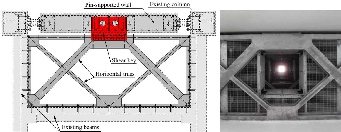
Figure 8. Horizontal connector.
