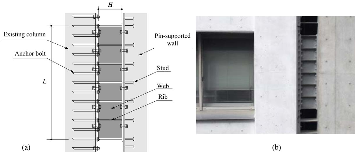
Figure 9. Completed steel damper with  $L = 1500$  mm.
